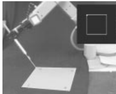
Figure 5: Mechanical pointing device used to assess the accuracy of our system
