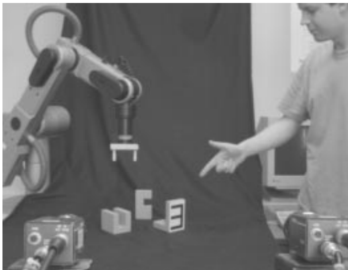
Figure 1.2: The experimental setup showing the robot, its workspace, stereo cameras and operator.
